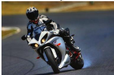
Tyre grip is not necessarily the same on each wheel. It varies with the load on the wheel and this affects the machine's balance and how it handles. Braking, changing direction and accelerating each alter the distribution of the load.
