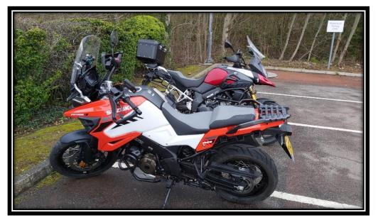
The 1050XT I was riding had wire wheels (spokes) but retained the standard 19-inch size, rather than going to the gyroscopic 21-inch. Despite the wire wheels being heavier than my cast ones, the front end of the 1050XT is much lighter.
