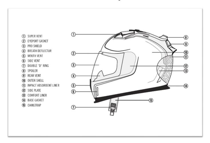
EPS liners are incredible pieces of technology (No.11 in the diagram). They are lightweight and work across a wide range of temperatures. Hot sunny days of +30 degrees and stuck in a freezing 70 mph wind that was -2 degrees when you were standing still.
