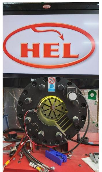
The machine applies 12 tonnes of pressure to the fixings to ensure an effective seal. Try as you might, you are never going to apply more pressure than the machine does.
