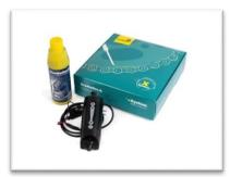
**xSystem** – Rather than being gravity fed, the xSystem has an electric pump and senses engine vibration, so it knows when to start pumping. It is arguably the simplest to install – not that the others are difficult. Connecting two wires to the battery is a task even I can manage. Once connected, you have a five flow rates plus a priming setting to choose from.
