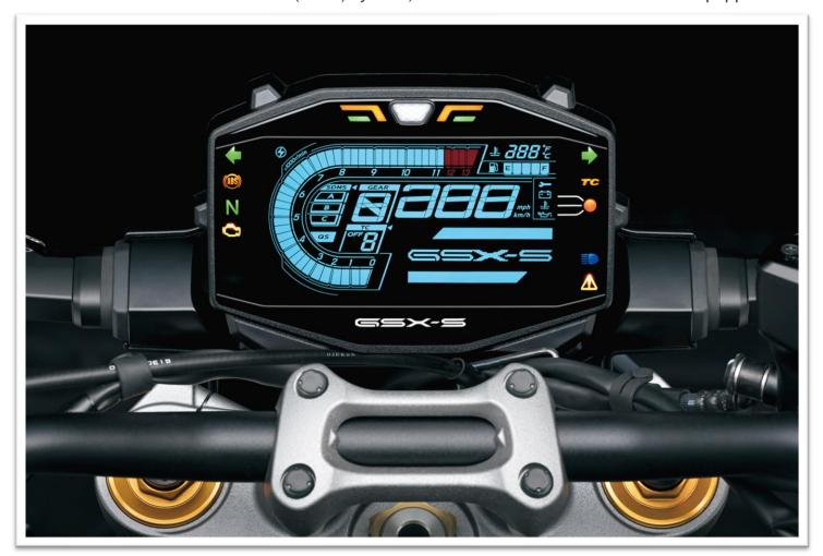
SDMS allows riders to choose from one of three engine maps, depending on the riding conditions or their own personal preferences. Modes A-C all deliver the same peak power, but vary the sharpness and immediacy of the delivery, with A mode the sportiest, and C mode delivering the softest power delivery.
