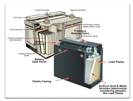
All batteries rely on a chemical reaction to generate electricity, which is why they eventually 'run out of juice' and cannot hold a charge any longer.
