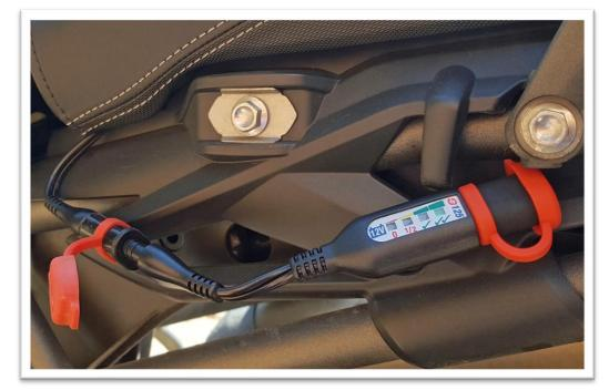
The battery was brought back to life with an Optimate 3 that can diagnose sulphation - crystals formed around the lead plates inside the battery, reducing performance - and automatically applied pulses of electric current to break the crystals down and recover the battery.
