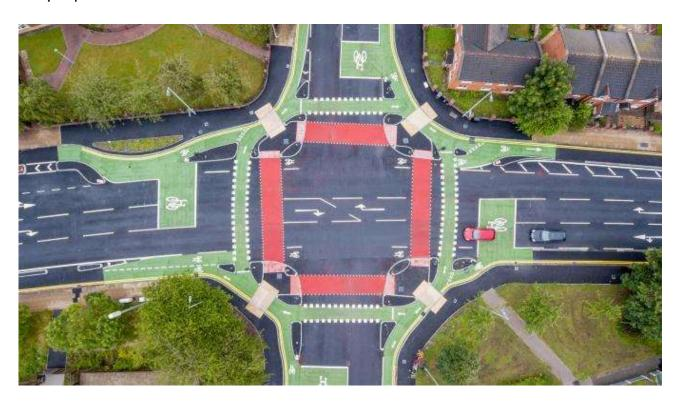
What is a CYCLOPS junction? CYCLOPS stands for Cycle Optimised Protected Signals. The unique design of the CYCLOPS junction completely separates pedestrians and cyclists from motor traffic at junctions, reducing the possibility of collisions or conflict.
